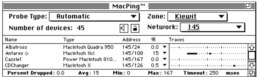
Figure 7. The MacPing window. This display shows that Albatross successfully answered all probes; CDChanger dropped one packet; Antares is no longer being tested because it dropped five packets in a row.
