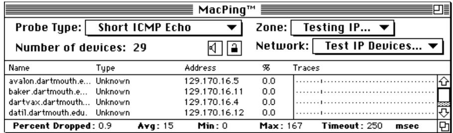
Figure 2. The MacPing window for testing IP devices.
