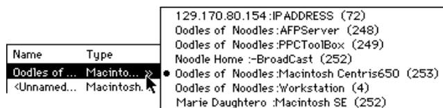
Figure 15. Device pop-up menu showing a node conflict. Notice that two different Macintosh types (Centris 650 and SE) are registered on a single network address.
